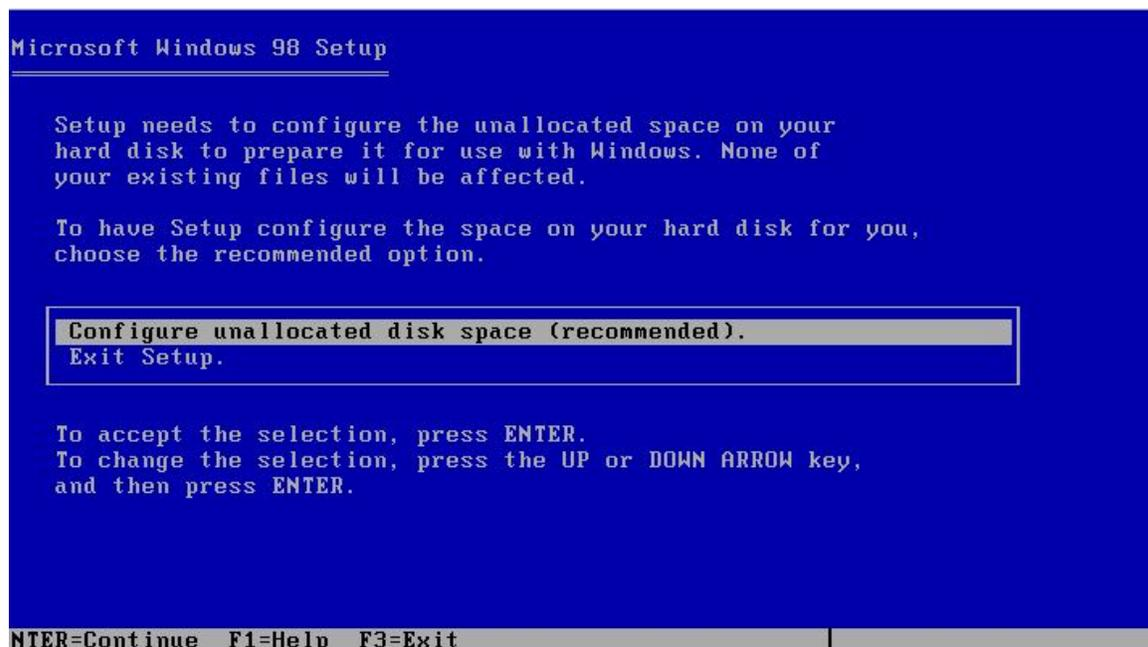
Select the option to configure the hard drive like in the top picture. Your system will restart. Repeat the operation to start the install. It will ask you to perform a system check (select OK) and then ask you to handle large hard drive. Select this option like in the below picture:
